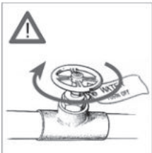
Wasserhauptahn absperrn Close the Main Water- Supply Valve
