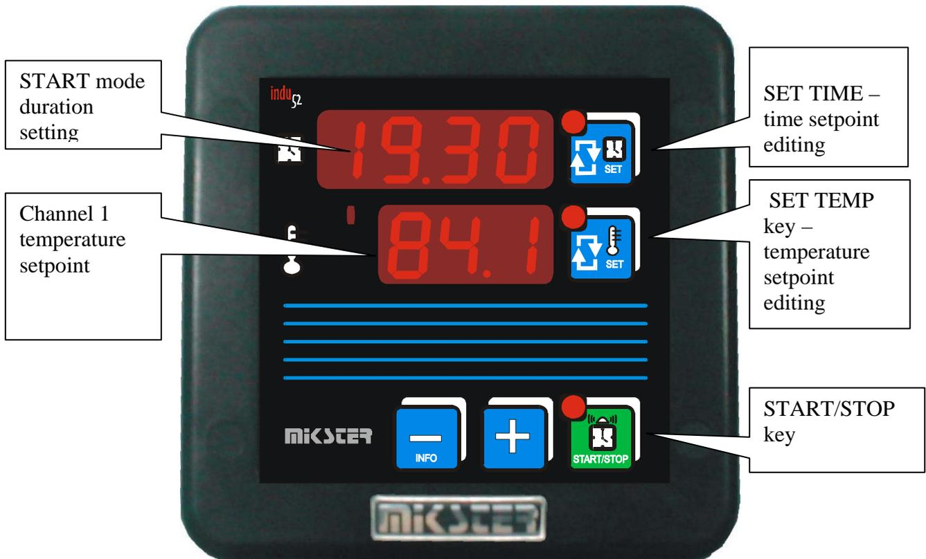
Fig: 1 INDU-52 Controller Front Panel
